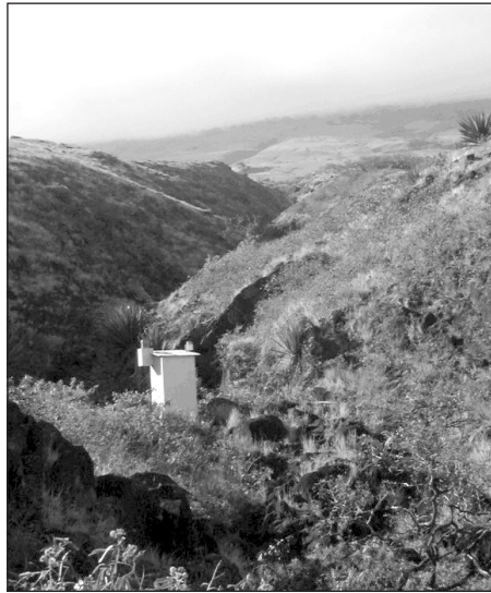
A USGS stream gage at Kepuni Gulch, Maui.
